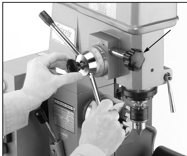
Figure 27. Move the handle while depressing knob.
